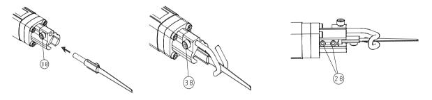
②Tighten the set bolts(28) as possible into the blade holder.
